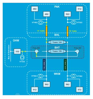
The normal configuration applies whenever PAK-WKM-1 and PAK-WKM-2 are in service and on completion of the repairs, from approximately 8/6/2026.
